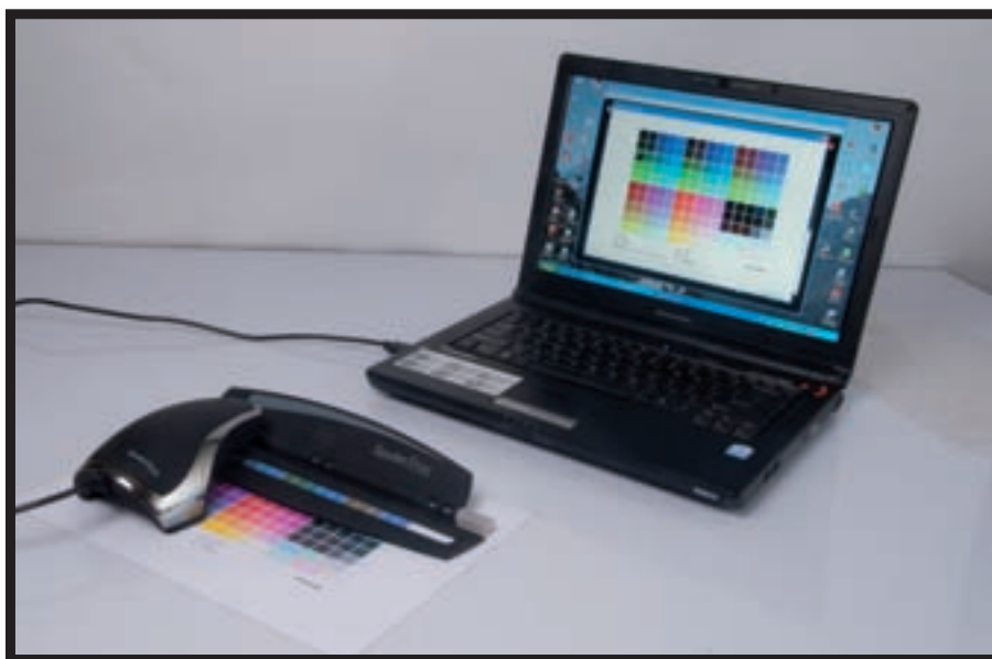
The Spyder colorimeter set up for calibration. The laptop screen shows the same set of colour patches as on the test print that is being measured
