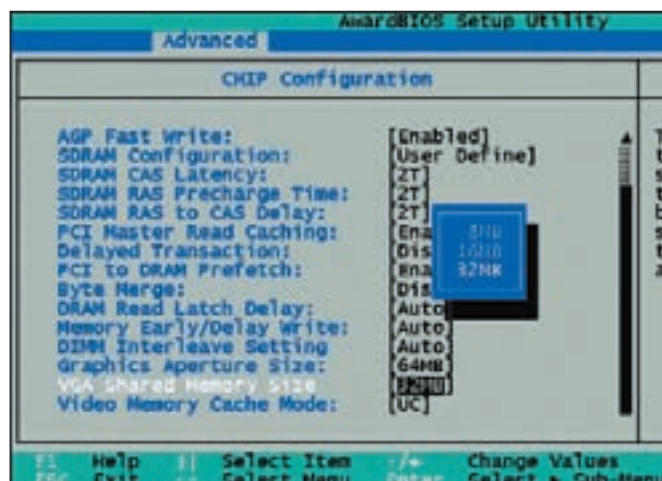
Memory allocated for the onboard graphics can be set in the BIOS
